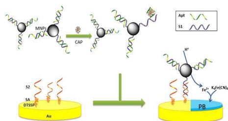
Fig. 1. Illustration of the procedures and detection mechanism of the proposed biosensor.
