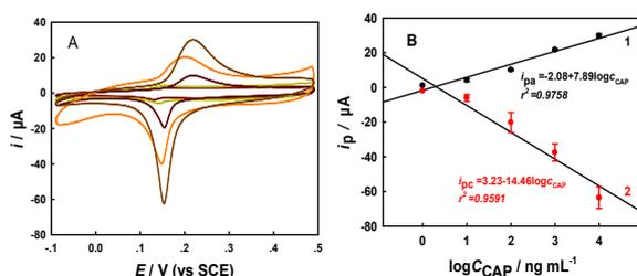
Fig. 5. (A) CV responses of biosensors to CAP at different concentrations (from top to bottom: control, 1, 10, 100, 1000, 10000 ng mL<sup>-1</sup>). (B) The calibration plot of oxidative (1) and reductive (2) peak currents to CAP concentrations.
