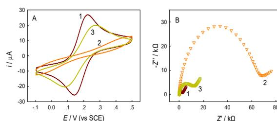
Fig. 4. CV (A) and EIS (B) of a bare gold electrode, MNPs-Apt-conjugated gold electrodes before and after ECC process (curves 1, 2 and 3 represent Au, Au-MNPs-Apt and Au-MNPs-Apt after ECC, respectively).
