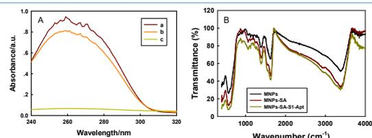
Fig. 2. (A) UV-vis spectra of the supernatants of the solutions before (a) and after (b) the aptamer conjugation, and the control (c). (B) FTIR spectra of three kinds of magnetic composites.
