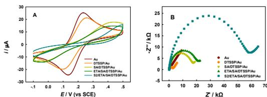
Fig. 3. CV (A) and EIS (B) of the layer-by-layer modification of electrodes.
